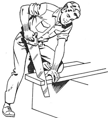
Fig. 14-13. Converting mechanical energy into heat energy.
