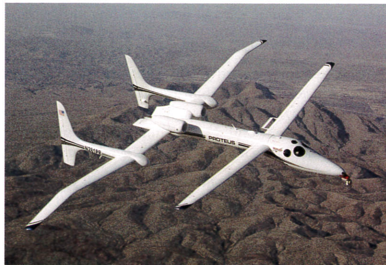
This NASA aircraft can fly up to 20 km above the earth’s surface. Atmospheric scientists have attached instruments to the bottom of the aircraft that can collect data on air temperature, water vapor, and air pollution.
