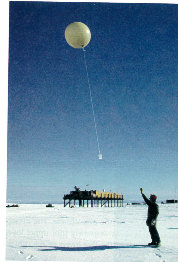
A researcher in Antarctica launches a weather balloon that carries a package of instruments to an altitude of around 25 kilometers.
